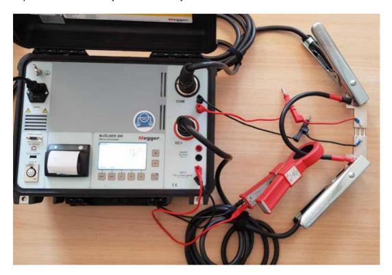
Turn on the power switch on the CT (make sure the batteries on the CT are charged). The LED shall lit.
